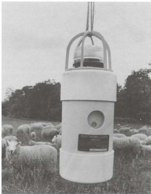
FIGURE 4. A siren-strobe device, developed by the Denver Wildlife Research Center, can effectively frighten coyotes away from sheep on bed grounds.
